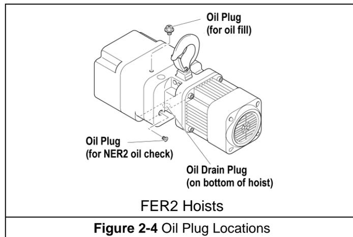
2.4.3 **REPLACING OIL** – Change gear oil at least once every 5 years. The oil should be changed more frequently depending on the hoist's usage and operating environment. See ER2 Owner's manual. Follow the procedure below for replacing the gearbox oil for your hoist:
