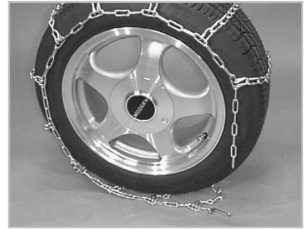
**3** Pull one cross chain down to the point where the tire meets the ground. Move the vehicle so that 1 or 2 cross chains pass under the tire.
