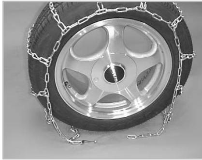
**2** Drape the chain over the tire, again making sure cross chain hooks are facing upward. Hooks that face down (towards the tire) will cause damage to the tire.
