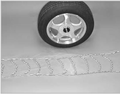
**1** Park vehicle on firm level ground and turn off the engine. Set the parking brake. Unroll the chains and lay them out flat making sure there are no twists or tangles. Make sure the smooth side of the cross chain hooks are toward the tire.
