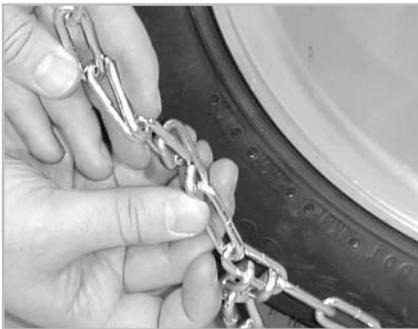
**4** Reach behind the tire and fasten the inside connector on the 2nd or 3rd link.
