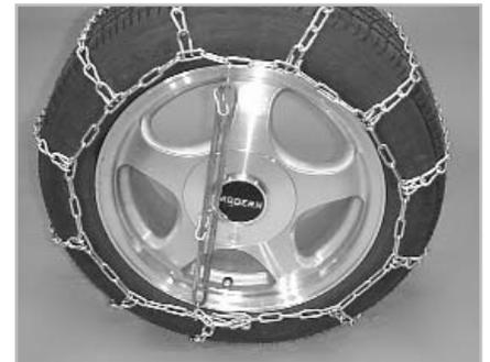
**6** Attach the rubber tensioner to take up the additional slack. To make this simpler, attach the first hook at the "5 o'clock" position and the second at the "11 o'clock" position and so forth. Tighteners must be purchased separately.
