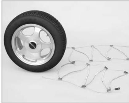
**1** Park vehicle on firm level ground, away from traffic and turn off the engine. Set the emergency brake. Remove any wheel covers. Chains should be installed on drive tires. Lay the cable chain on the ground with the smooth side (TIRE SIDE) of the cross member hooks up.
