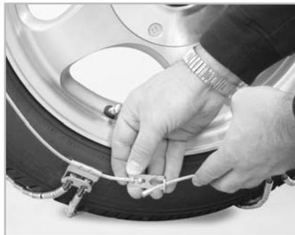
**5** Take the bushing end of the lower fastener and thread it through the keyhole (the one near the ground) using the same process as the top fastener. Please see below for a detailed look at making this connection.
