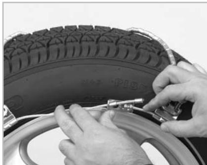
**4** At the top of the outside cable, take the bushing end of the outside split side cable and thread it through the keyhole fastener. Grasp the outside cable with both hands and pull it toward you to create as much slack as possible.
