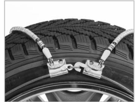
**3** Reach around each side of the tire and grasp both ends of the non-split cable (the cable that is furthest away from you). Pull both ends to the top of the tire so the fasteners can be seen and manipulated more easily. Connect the inside fastener.
