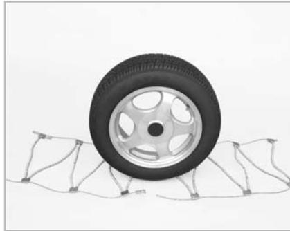
**2** Move the chain in a sweeping motion under the vehicle so the open mid-section is positioned against the backside of the tire. This sweeping motion can best be done while kneeling in front of the tire.
