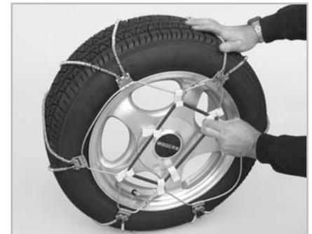
**6** Attach the rubber tensioner to take up the additional slack. To make this simpler, attach the first hook at the "6 o'clock" position, the next at the "12 o'clock" position and so forth. The open side of the hooks must face away from the tire. No further adjustment is necessary.
